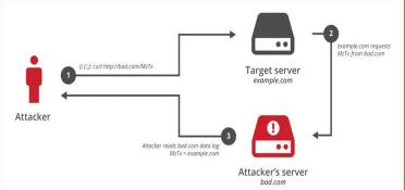
Another technique that have been used to identify vulnerable servers is to make the web server download a web page from an attacker-controlled machine. The attacker can then look in their web server logs to find out which machine was vulnerable. This attack works by sending the following Shellshock string:
